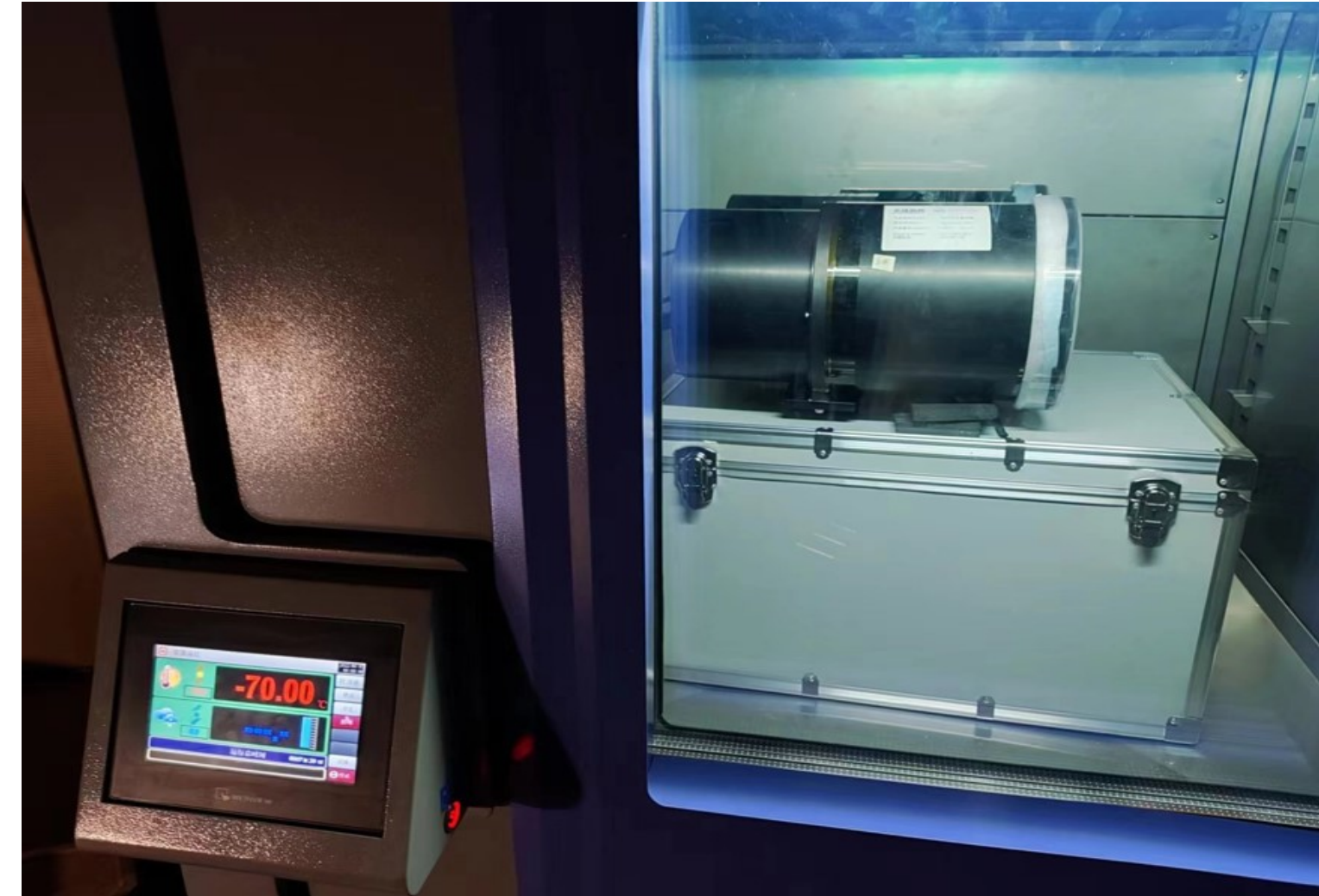
Figure 3: We tested the cold start and hot run-ning of the equipment in a cryogenic chamber.
